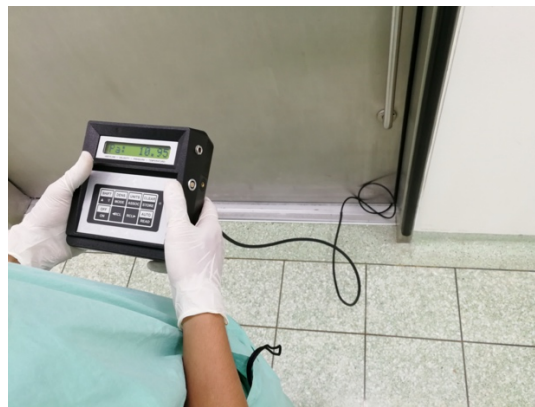
Figure 3 – Measuring Air Pressure to Verify Seal Integrity
